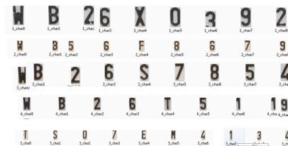
Fig. 2. Segmented character using OpenCV
