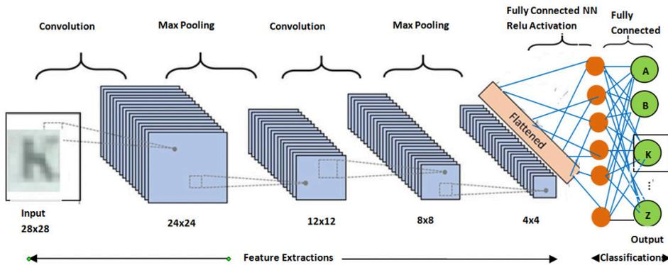
Fig. 3. Convolution Neural Network Model to recognize number plate image
