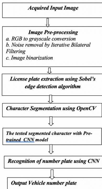
Fig. 1. Basic steps for Automatic Number System Recognition
